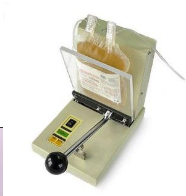
It detects RBC to clamp tubing immediately.
